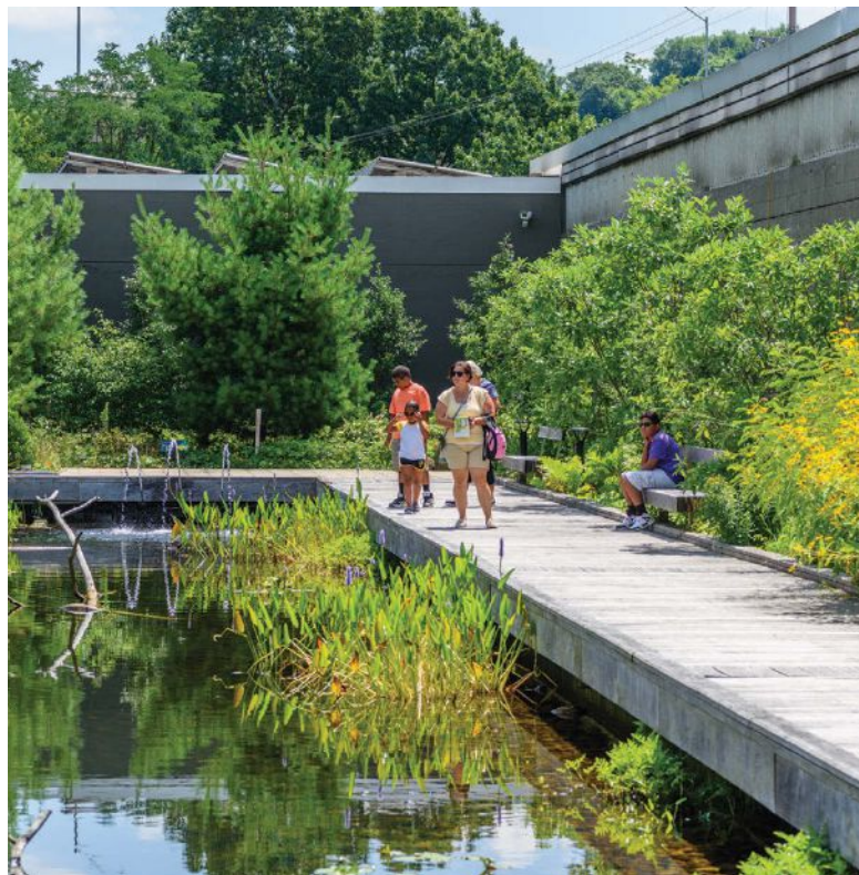
Left: Turtle Lagoon not only is an important visitor amenity at Phipps, it also helps manage all the stormwater over three acres. Right: The energy-efficient Tropical Forest Conservatory is 100 percent passively cooled and has no greenhouse effect.
